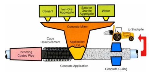
Figure 4.5 Concrete-coating process.
