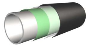
Figure 4.3 Three-layer polyethylene (3LPE) external anticorrosion coating principle. The coating consists of an inner layer of fusion-bonded epoxy (dark green), an adhesive layer in the middle (light green) and a top layer of polyethylene (black).
