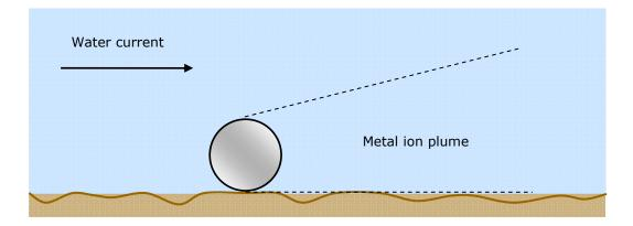
Figure 5.3 Principle in the simplified advection-dispersion model used for estimation of the spreading of zinc from the anodes.
