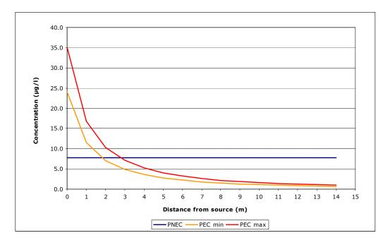
Figure 5.4 Relationship between PEC and PNEC for zinc released from a zinc anode.
