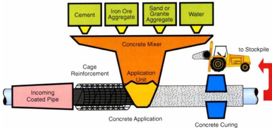
Figure 4.5 Concrete-coating process.
