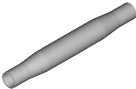
Figure 4.1 Buckle arrestor principle. The buckle arrestor has a greater wall thickness than the adjacent section of pipeline.
