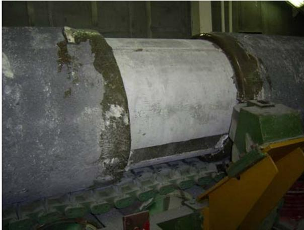
Figure 4.8 A sacrificial anode is mounted in a gap in the concrete coating and directly attached to the pipe.
