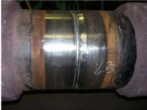
Figure 4.6 A typical field joint before coating. The three-layer polyethylene anticorrosion coating and the concrete coating are visible on the line pipes.
