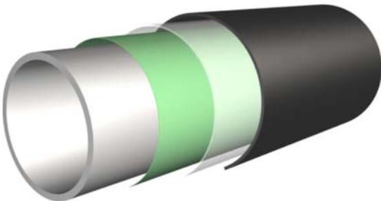
Figure 4.3 Three-layer polyethylene (3LPE) external anticorrosion coating principle. The coating consists of an inner layer of fusion-bonded epoxy (dark green), an adhesive layer in the middle (light green) and a top layer of polyethylene (black).
