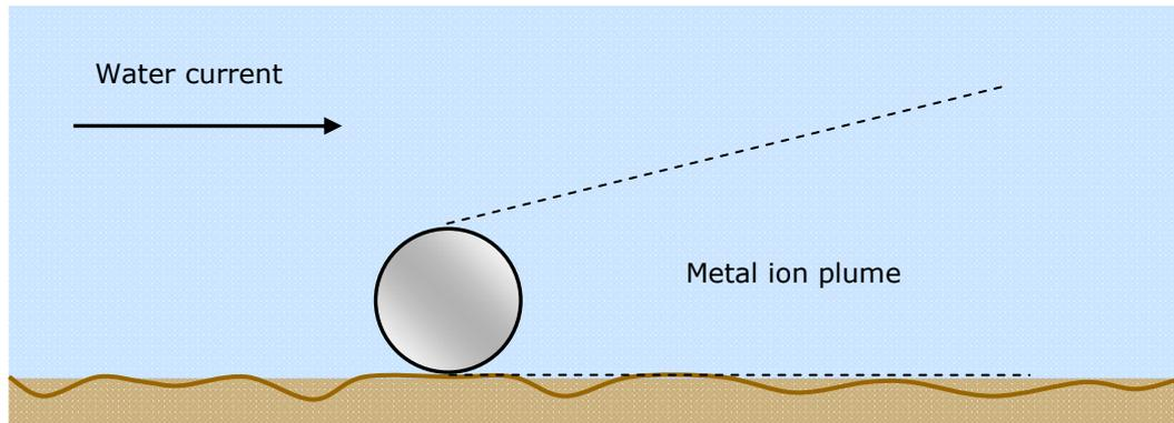
Figure 5.3 Principle in the simplified advection-dispersion model used for estimation of the spreading of zinc from the anodes.
