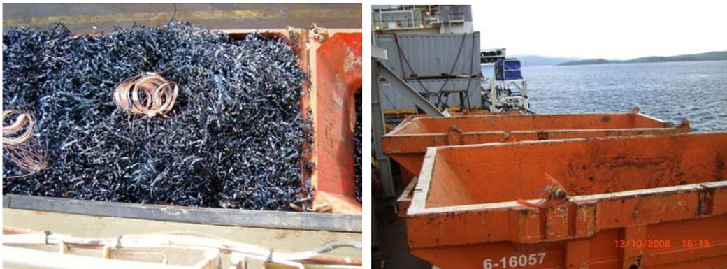
Figure 5.1 Metal scraps from the bevelling process (left) and typical containers (right).
