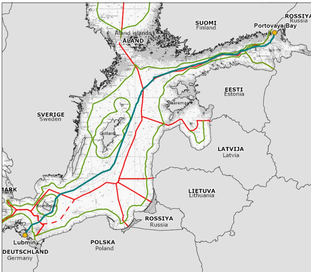
Figure 3.1: The Nord Stream pipeline route through the Baltic Sea. The dark green line indicates the pipeline route. The red lines indicate the exclusive economic zones of the countries around the Baltic Sea, and the green lines indicate the limit of the territorial waters. The dotted red line indicates the midline between Denmark and Poland.
