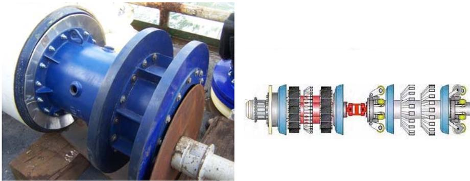
Figure 5.2 Examples of 'pigs'. A gauge pig being pushed into a pig launcher (left) and drawing of a typical intelligent pig for internal inspection (right).
