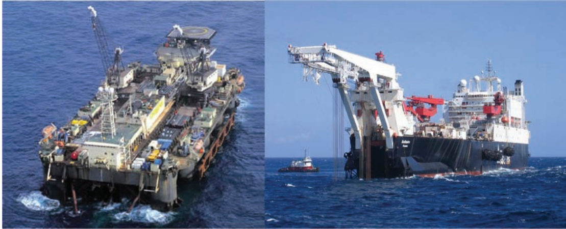
Figure 0.6. Pipe-laying barges Castoro Sei (left) and Solitaire (right).
