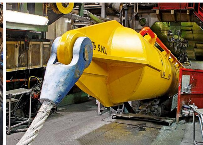
A cable is attached to the end of the PIG launcher. With its help, the pipeline is lowered to the seabed. Once the pipeline is positioned, the cable is released.
