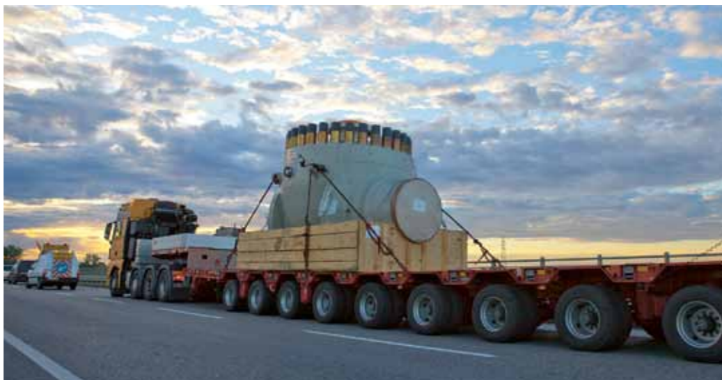
Transporting 100 tonne components on the road across Europe requires thorough planning and special approvals.
