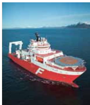
The Far Samson is 121.5 metres long, 26 metres wide, and can carry up to 6,130 tonnes.
