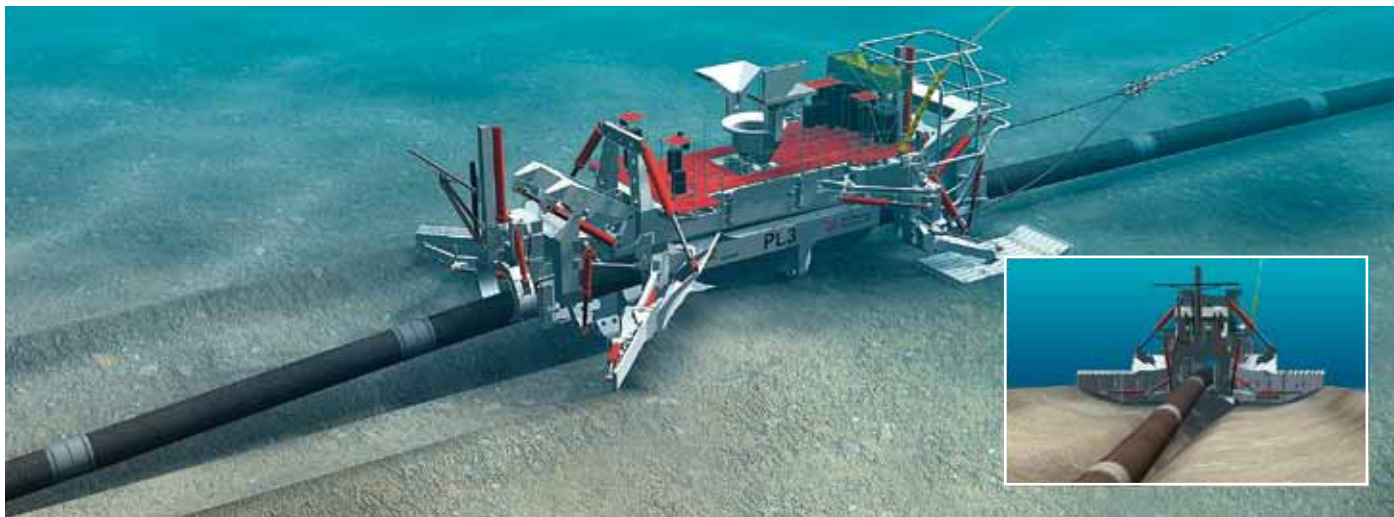
The PL3 raises the pipeline into its roller boxes, and is then towed by the Far Samson creating a trench into which the pipeline is laid as the plough moves forward.
