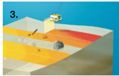
3. In 2007 and 2008 a 25 metre corridor for each pipeline was inspected with high resolution equipment. Potentially dangerous objects were evaluated by independent experts.
