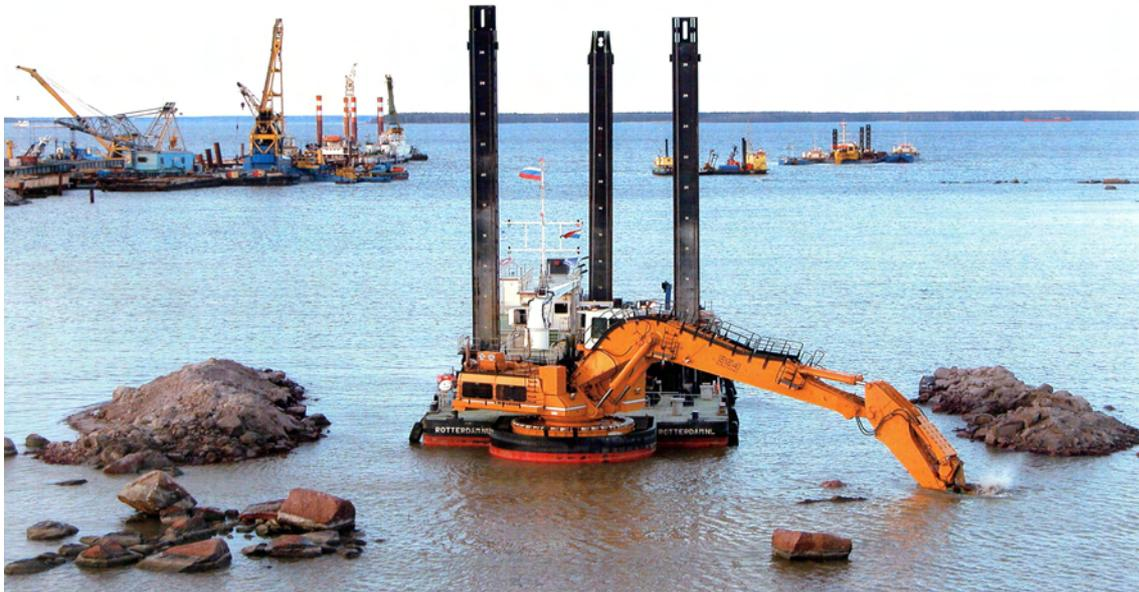
**Figure 3.1** Hydraulic backhoe dredger mounted on a pontoon
