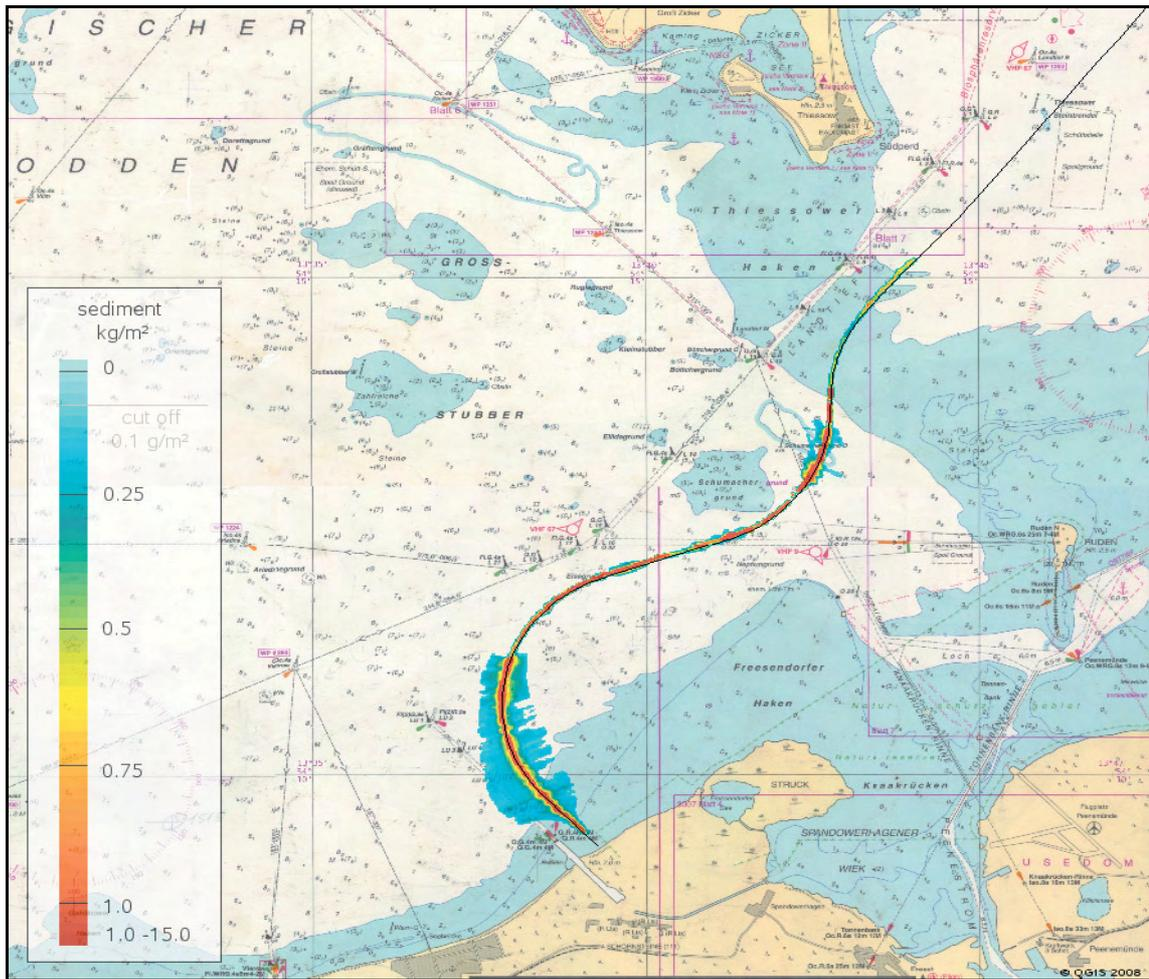
**Figure 4.8 Summary of sedimentation rates (in  $\text{kg/m}^2$ ) for all wind directions with a wind speed of 5 m/s and an interference interval of 5 days**
