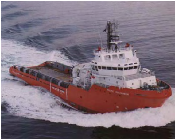
Figure 2.3 Anchor handling tug
