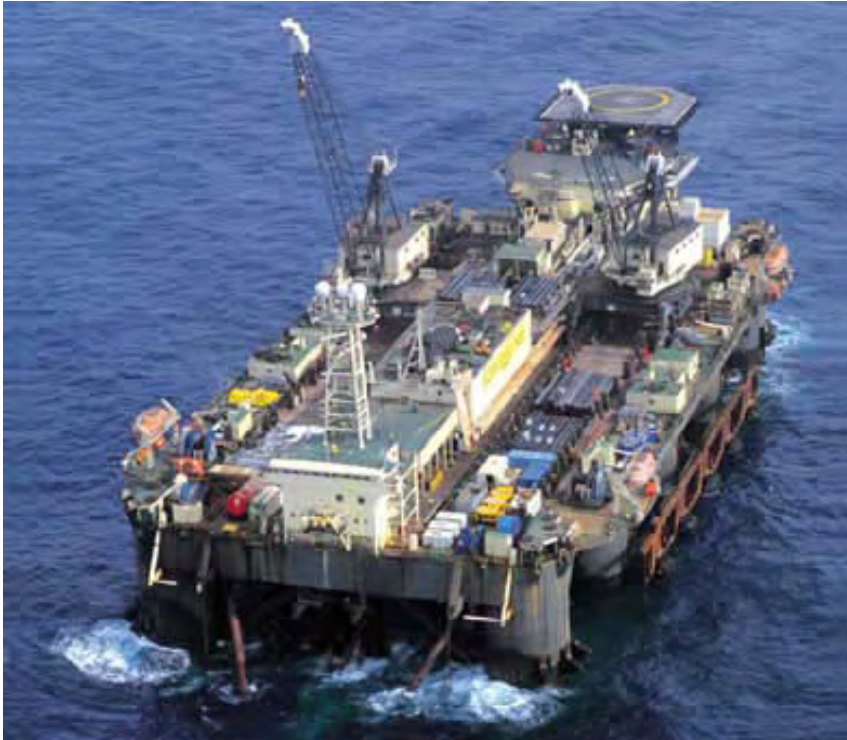
Figure 2.2 Castoro 6 pipe-lay barge
