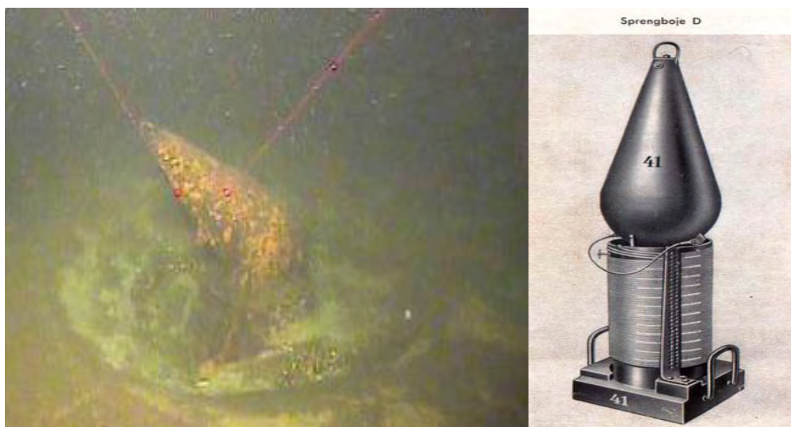
Figure 2.22 Target R-09-04, WWII Mine line anti-sweep explosive device, conical casing with rounded base resting on the possible remains of its deployment system in a scoured hollow on a seabed of sandy clay. Identification: SPB D German Obstructor Mine, Charge 0.8 kg, External features push / drag sensor
