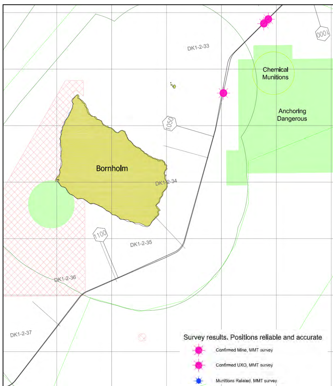
Figure 2.18 Munitions found in the Danish project Sector within 25 m of the Nord Stream pipeline routes (C16)
