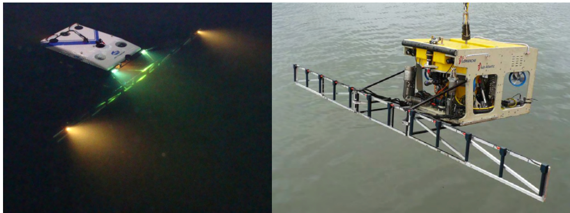
Figure 2.11 ROV-mounted gradiometer array: Russian Sector (left image), Finnish, Swedish, Danish and German Sectors (right image)
