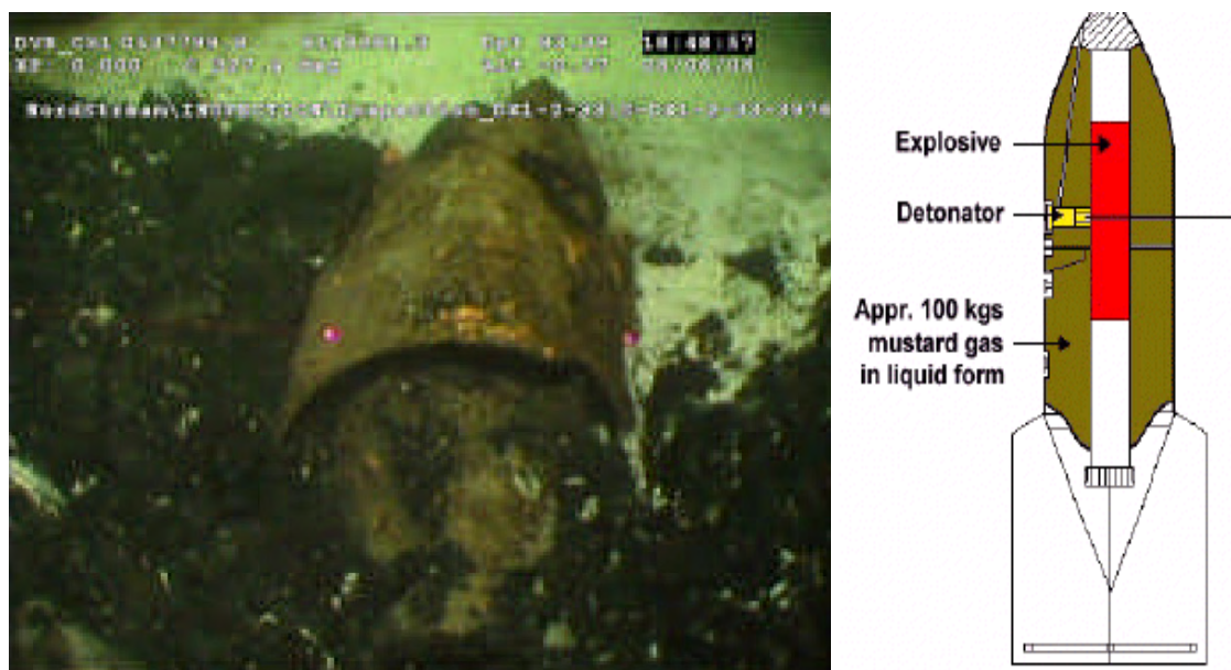
Figure 2.23 DK1-2-33-3976, WWII A German chemical 250 mustard gas bomb. The casing is heavily corroded and the some of the gas is still in the bomb, approx up to 30 kg.
