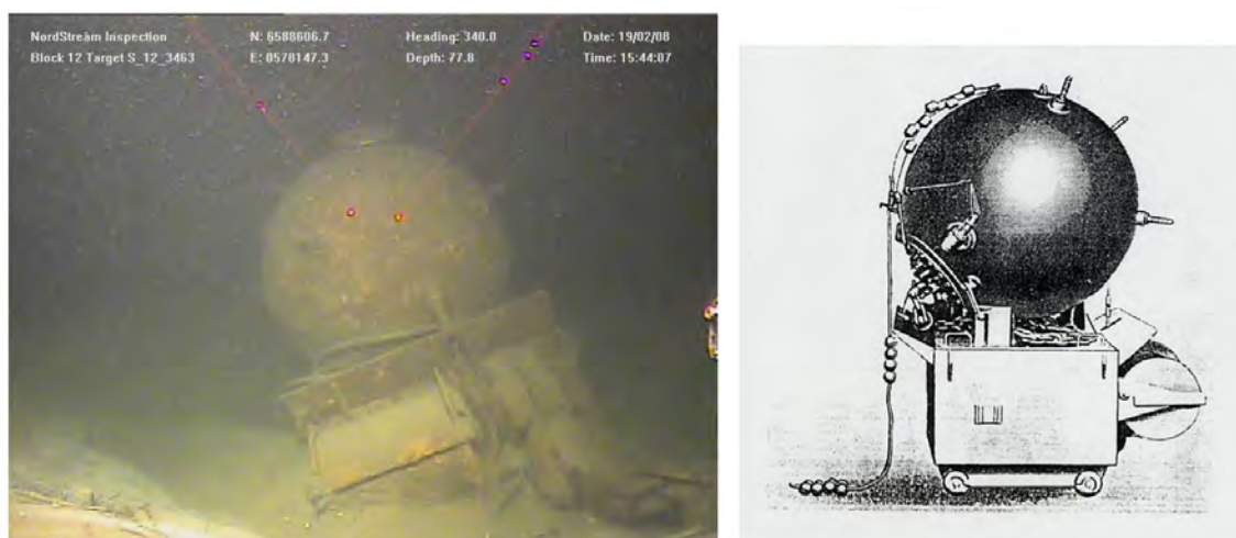
Figure 6.1 Correlation of munitions survey findings with historical records. The image on the left shows a mine with an anchoring mechanism that is located in a deep, scoured hollow surrounded by a flat seabed of soft gyttja clay. Based on the drawing on the right, the object has been identified as an EMC I + II German WW II moored contact mine, with either a 250 kg or 320 kg hexanite charge
