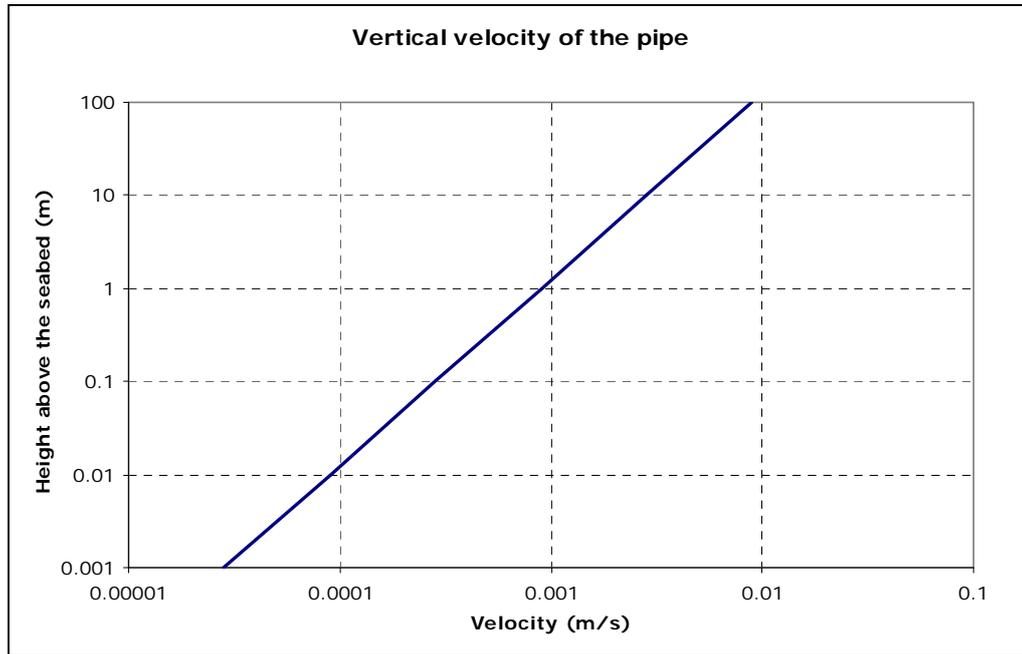
Figure 3.1: Vertical velocity of the pipeline in the water column during pipeline layout
