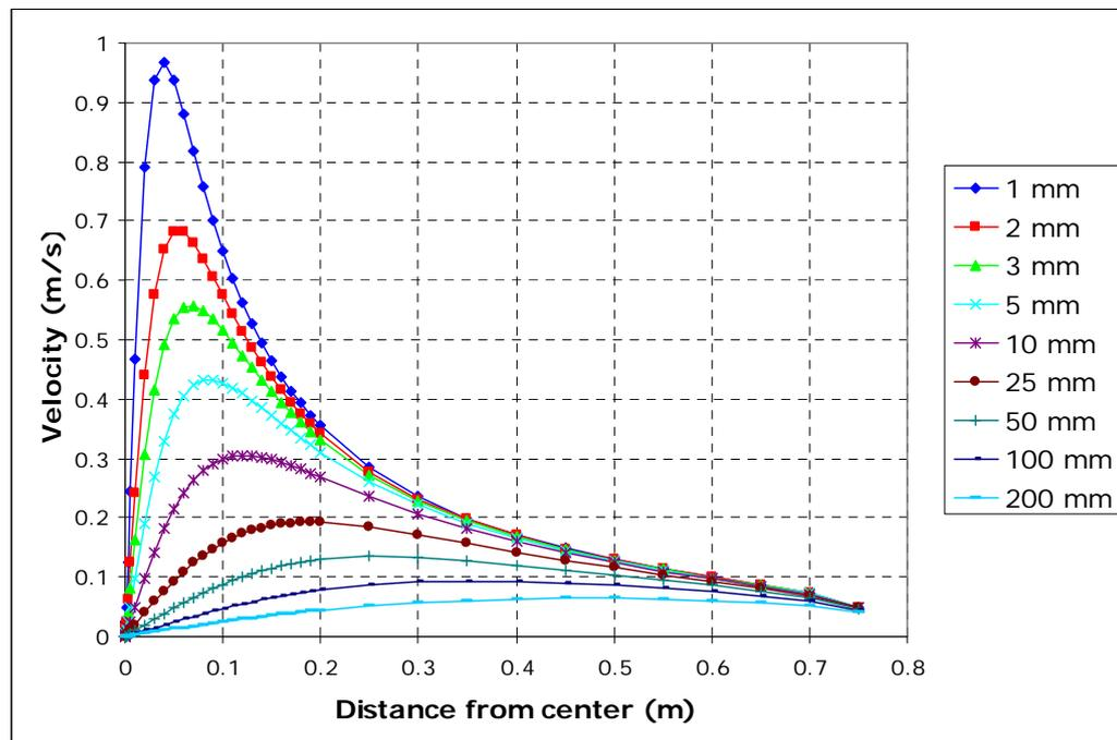
Figure 4.1: Horizontal flow velocity below the pipeline for a vertical pipeline velocity of 5 cm/s. This is valid for the lay barge under rough conditions.
