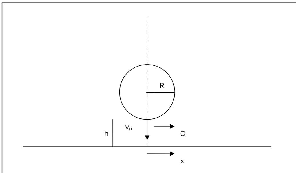
An approximation to the flow velocity can be reached by calculating the mean velocity of the displaced water volume flowing out in the area below the pipe. The volume of water that has to escape below the pipe per time unit is zero below the centre of the pipeline and increases towards the edges of the pipe, with an equal flow on each side of the centreline. Anticipating a constant downwards velocity of the pipe, the flow as a function of the distance from the centreline is given by:
