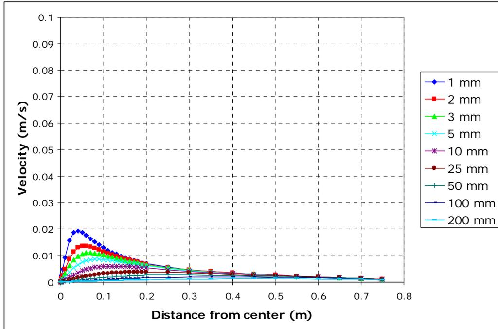
Figure 4.2: Horizontal flow velocity below the pipeline for a vertical pipeline velocity of 0.1 cm/s. This is valid for the lay barge under calm conditions.
