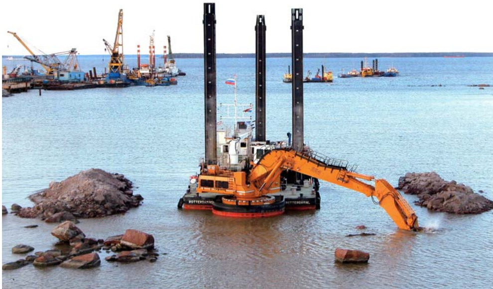
Figure 3.6 The scoop dredger “At Your Service” of the company MPTC, /24/.
