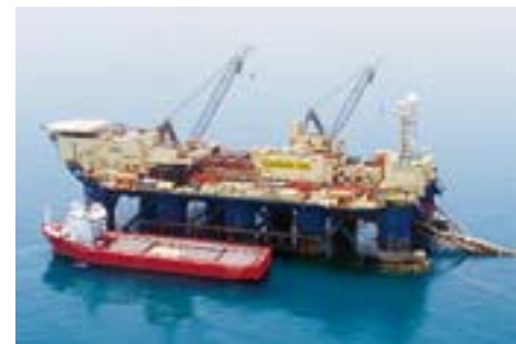
The pipeline is lowered to the seabed from a pipelay vessel. Up to 3 kilometres can be built each day.
