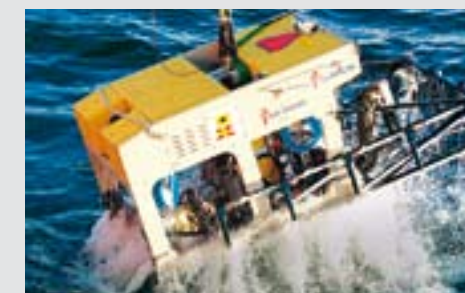
A high-tech ROV is deployed from a research vessel to screen for munitions.
